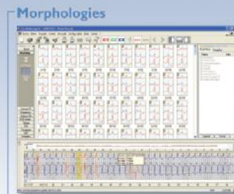
It displays the analysed forms, divided in groups: Normal, Ventricular, Pacemaker, Others and Artifacts. It allows users to edit forms that are preselected by the system.
